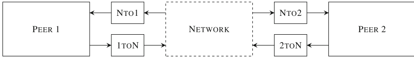
Fig. 5. TCP threat model block diagram. Each box is a process. An arrow from process P_1 to process P_2 denotes that a subset of the outputs of P_2 are exclusively inputs of P_1 . PEERS 1 and 2 are TCP peers. A channel is a directed FIFO queue of size one with the ability to detect fullness. A full channel may be overwritten. 1TON, NTO1, 2TON, and NTO2 are channels. Implicitly, channels relabel: for instance, 1TON relabels outputs from PEER 1 to become inputs of NETWORK; NETWORK transfers messages between peers via channels, and is the vulnerable process.
